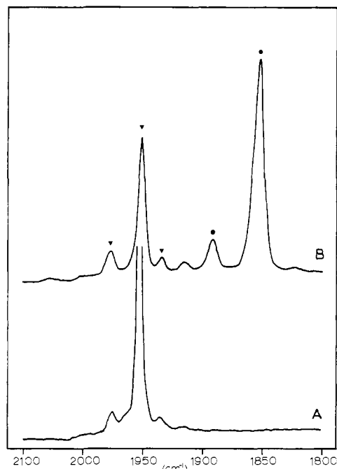
Figure 2. IR spectra following the photolysis of \text{Mn}_2(\text{CO})_8[\text{P}(i\text{-Bu})_3]_2 with \text{P}(i\text{-Bu})_3 in hexane: (A) initial; (B) after several hours photolysis. The absorptions are assigned as follows: (▼) to \text{Mn}_2(\text{CO})_8[\text{P}(i\text{-Bu})_3]_2 ; (■) to \text{HMn}(\text{CO})_3[\text{P}(i\text{-Bu})_3]_2 ; (●) to \text{Mn}(\text{CO})_3[\text{P}(i\text{-Bu})_3]_2 .
